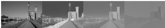
Figure 6: RGB-NIR opponent colour components of a scene. The colour transformation converts colour differences into spatial patterns, which are well characterised by local descriptors such as SIFT. Note that there is visibly less energy in the later components.
